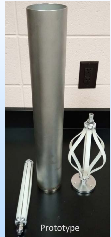
Horizontal tensor strainmeter (nested areal) Closed downhole package
